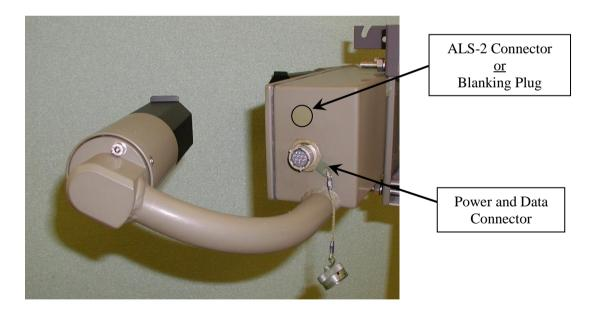
Figure 1-2 Cable Connectors
