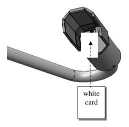
Figure 4-1 Transmitter hood with white card
