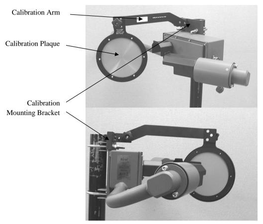
**Figure 5-1 Calibration Plaque Mounting Details**
